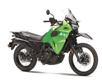
instrumentation panel, high-tensile double-cradle frame, and LED headlight. For 2023, the KLR650 S receives lowered front and rear suspension with dedicated settings that help enhance the rider's reach to the ground yet retain the excellent handling and comfort characteristics of the KLR650. Accompanying the lower suspension settings is a new low seat, updated shifter-to-footpeg distance, and shorter side stand.
