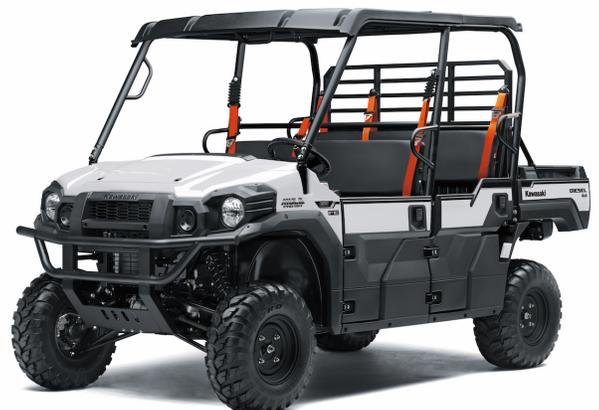
Each MULE PRO side x side is built with a tough chassis that provides a smooth ride through the use of independent suspension front and rear. The suspension provides a generous 8.7" of travel and excellent ground clearance. The entire MULE lineup is built to be the hardest worker on the job site.
